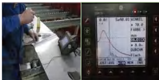
臂架100%UT探伤 100% UT flaw detection for boom
